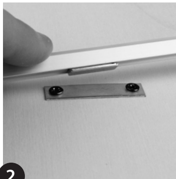
Attach magnets to steel plates.
